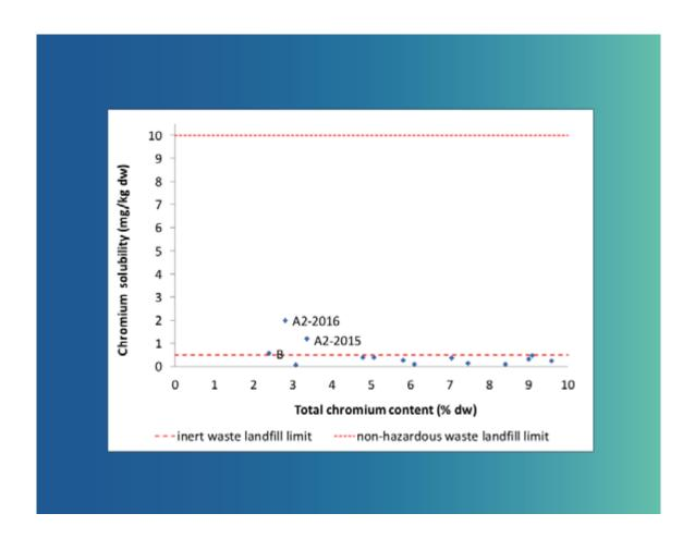
Eleven out of the fourteen tested FeCr slag samples during 2015-2016 met the requirements for inert waste (0.5 mg/kg), even at high total chromium contents. All samples met the requirements for non-hazardous waste landfills (10 mg/kg).
