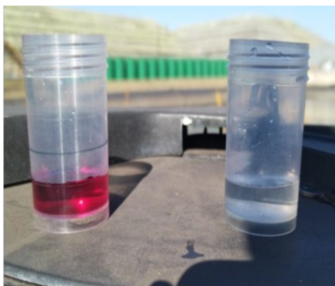
Chemical analysis indicating complete removal of hexavalent chromium
